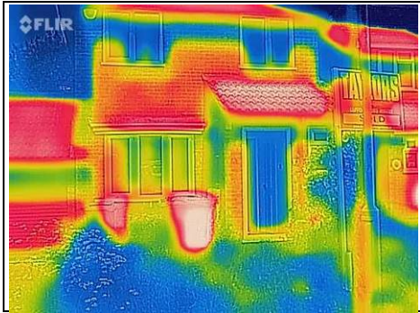
Example thermal image with the red areas showing the warmth of the sun (Not your property)
