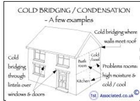
Cold bridging / thermal bridging
