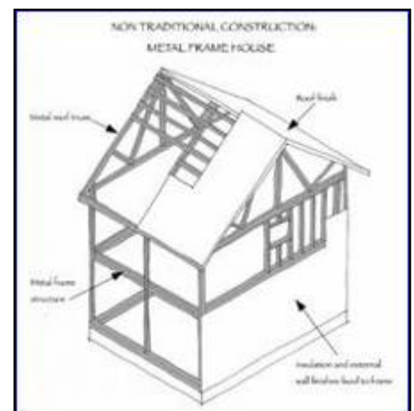
Metal frame non traditional construction
