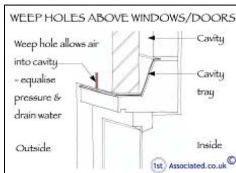
Weep holes above windows
