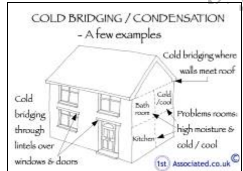
Cold bridging / thermal bridging
