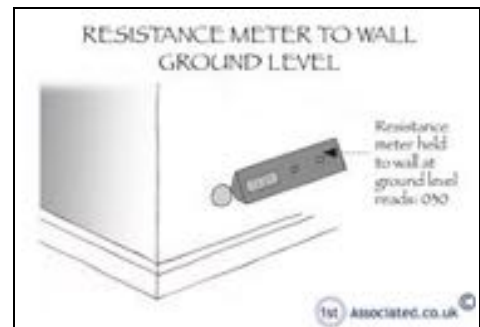
Testing for rising damp
