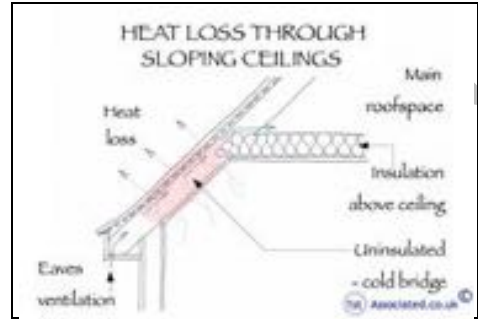
Heat loss through sloping ceilings
