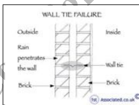
Wall tie failure
