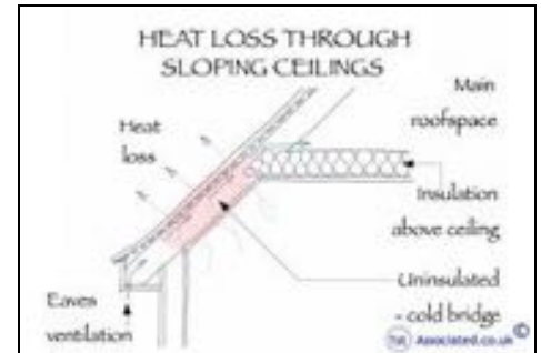
Heat loss through sloping ceilings
