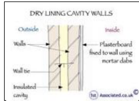
Cavity walls insulated
