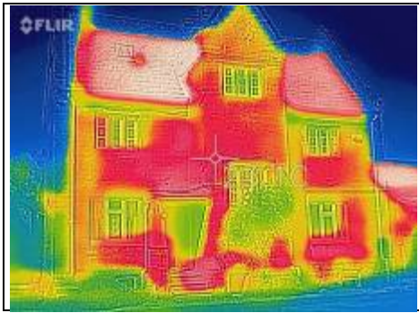
Front of house, property warmed up by the sun (not your property)
