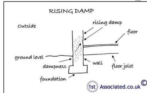
A random visual inspection and tests with a moisture meter have been taken to the perimeter walls and some internal walls. The readings we obtained indicated that there is dampness in the property which we were not surprised at, particularly the front wall which from what we can see has all the rainwater discharging on it from the adjoining car park. We will not be at all surprised if there is damage and deterioration to the timbers to this elevation.
