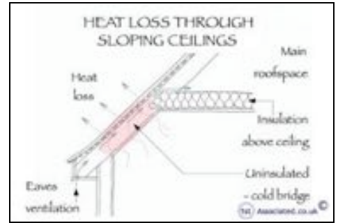
Heat loss and sloping ceilings
