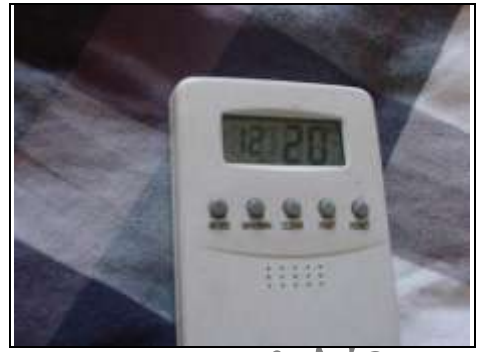
Relative humidity readings of 20% in the master bedroom
