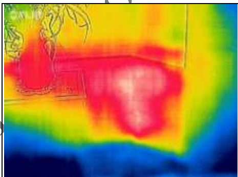
Heat loss through external bay walls
