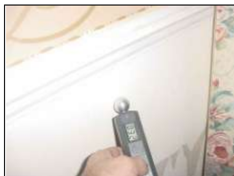
Taking lateral damp meter readings
