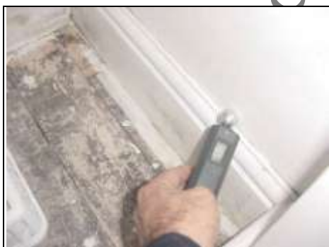
Taking rising damp meter readings
