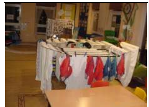
Drying clothes internally adds to humidity
