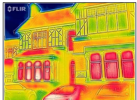
Front of property showing energy coming through windows and doors and from main roof
