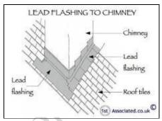
Lead flashing to replace cement flashing
