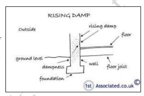
A visual inspection and tests with a moisture meter have been taken to the perimeter walls. In this case we have found rising damp particularly to the left hand side.
