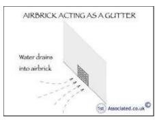
Air brick unprotected allows water in
