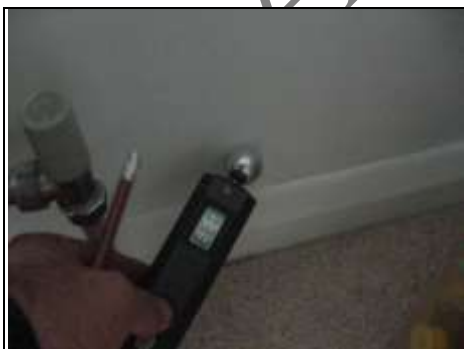
Testing for rising damp
