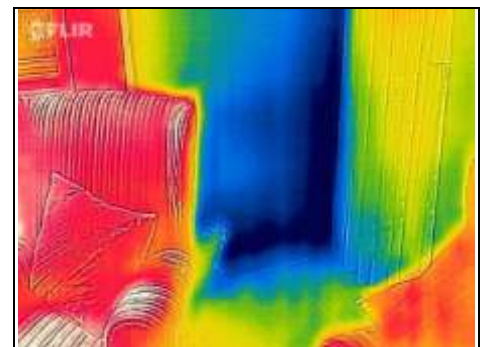
Thermal imaging photo of lounge – both walls colder than we would expect
