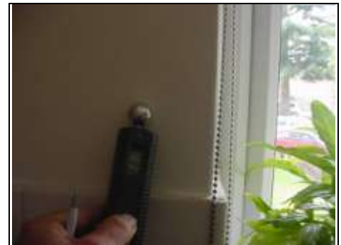
Testing for lateral dampness
