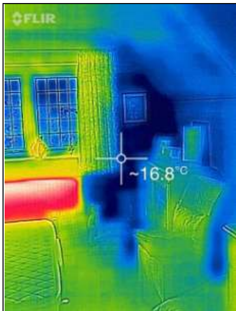
Thermal image Colder walls in upstairs bedroom
