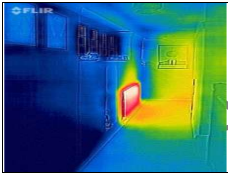
Heating test (red is radiator, blue is coldness of wall)
