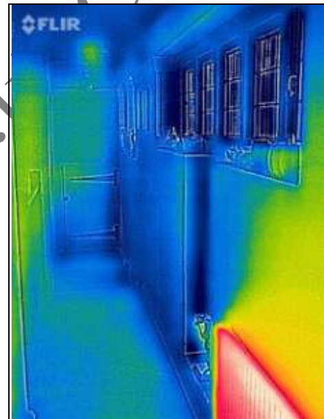
Thermal image Cold walls to first floor landing
