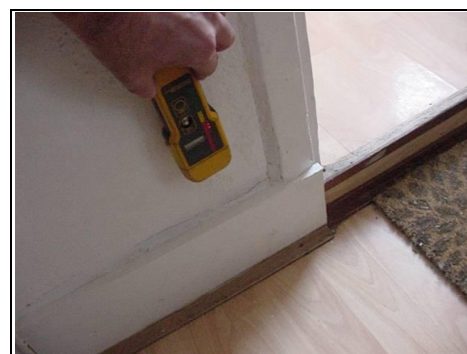
Testing and finding rising damp
