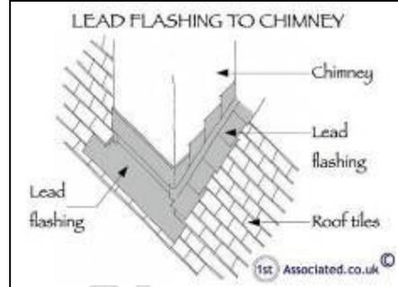
Lead flashing to replace cement flashing
