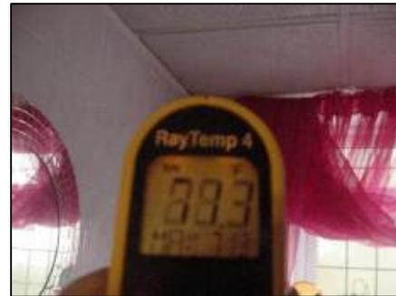
Surface temperature reading at the top of the wall is 77
