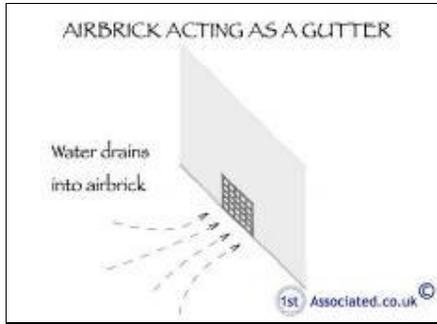
Air brick unprotected allows water in
