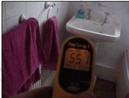
Surface temperature reading at the bottom of the wall is 55
