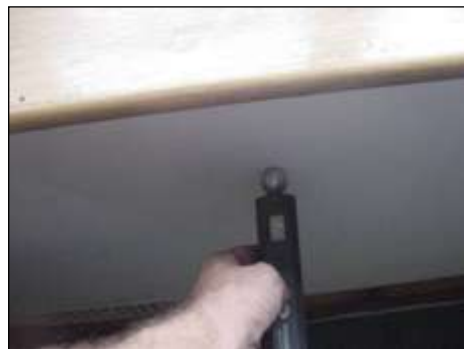
Testing for dampness and showing it is dry lined
